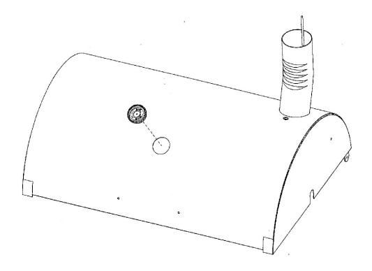
Attach grill lid handle (item #23) using two M6 x 15mm Phillips head bolts and M6 hex nuts.
